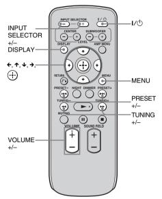
Press INPUT SELECTOR + or – repeatedly until "FM" or "AM" appears in the front panel display.
